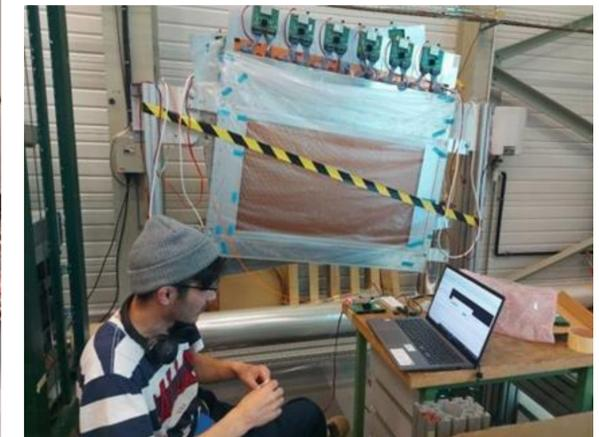
Straw detector setup for NA64 2022B run includes 3 station of small chambers and one station of large chambers, each station has 2 chamber of straw detectors. Picture of small chambers(left) and picture of large (UV) straw chamber(right)
