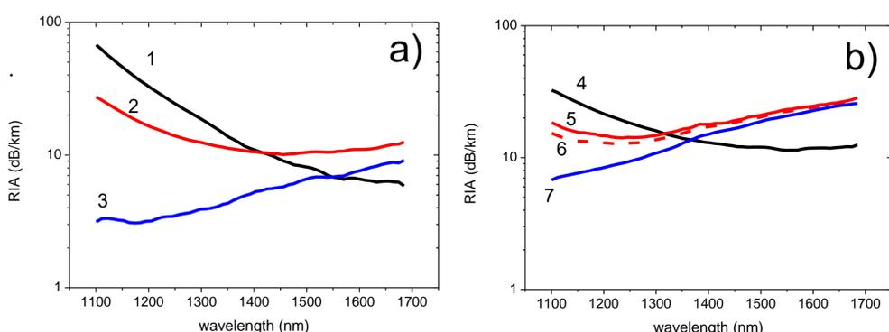
Fig 4. a) RIA spectra during irradiation and relaxation at I stage of irradiation (points 1 - 3.7 kGy, 2 - 82 kGy, 3 - 30 min of relaxation after 82 kGy), b) - at II stage of irradiation 4 - 82.5 kGy, 5- 479.7 kGy, 6 - 480.2 kGy, 7 - 15 min of relaxation after 590 kGy). Temperature  $T=25$  °C for spectra 1-5 and  $T=40$  °C for spectra 6-7
