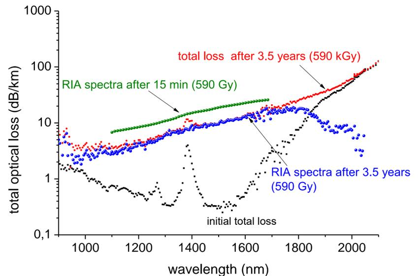
Fig 5. Spectrum of optical loss. Initial loss (black dots), loss 3.5 years after irradiation with a dose of 590 kGy (red dots), RIA spectrum after 15 min (green dots) and 3.5 years (blue dots) after irradiation
