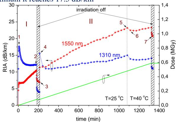
Fig 3. RIA and dose (green curve) evolution with time of irradiation and post-irradiation recovery at wavelengths 1310 nm (red curve), 1550 nm (blue curve).
